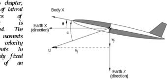
aircraft system are shown in Fig (2) where the aerodynamic moment components are represented by L, M and N the angular rate components of roll, pitch and yaw axis are represented by p, q and r and the terms u, v and w represents the velocity components of roll, pitch and yaw axes. Transfer function for rudder deflection angle to yaw angle is given by equation
