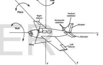
vertical axis, and rotation with reference to this axis is called yaw.
